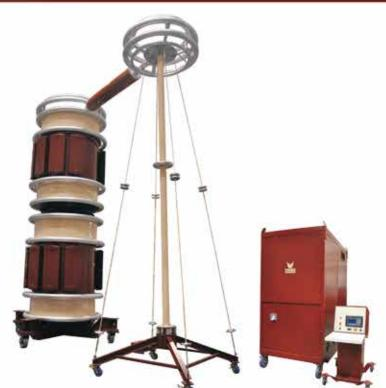
AC, Cascade Type, 400 kV, 800 kVA
